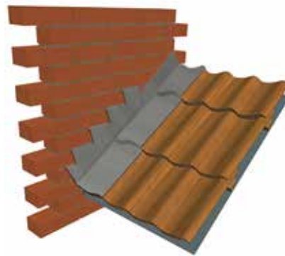
Figure 07: flashing to a side abutment – single lap tiles
